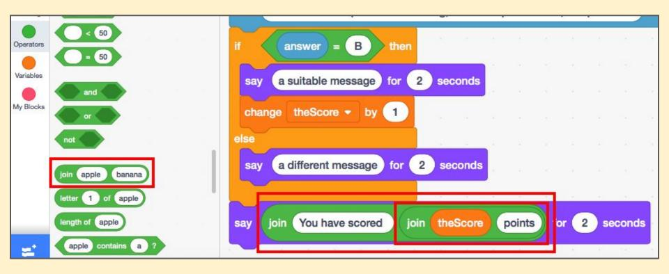
Adding a complex message can be done by using a **join block** (or two)
